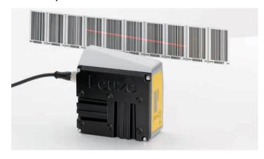
The FBPS 600i works particularly reliable. Each scanning operation reads several codes from which the software determines highly precise position values. The diagonal path of the scanning beam and the movement of the device mean that each code is scanned at different points. This prevents reading errors caused by local soiling or damage.
