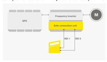
The FBPS 600i requires just one sensor for safe position detection. The device is connected to a safe evaluation unit – e.g. a frequency inverter – via two SSI interfaces. Furthermore, the devices already meet the requirements for PL e / SIL 3. As a result, safety functions can be implemented extremely easily and the time and effort required for installation and servicing is reduced.
